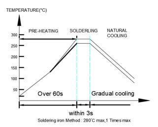
Soldering iron method: 280°C Max
